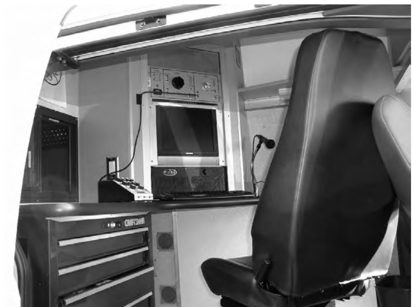
Top: Digital photo of a cracked sewer pipe as captured during Closed-circuit television (CCTV) inspection. Bottom: Operator control room inside CCTV inspection van.
